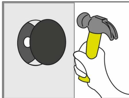
Position fixing covers and push in to place with a hammer x 4.
