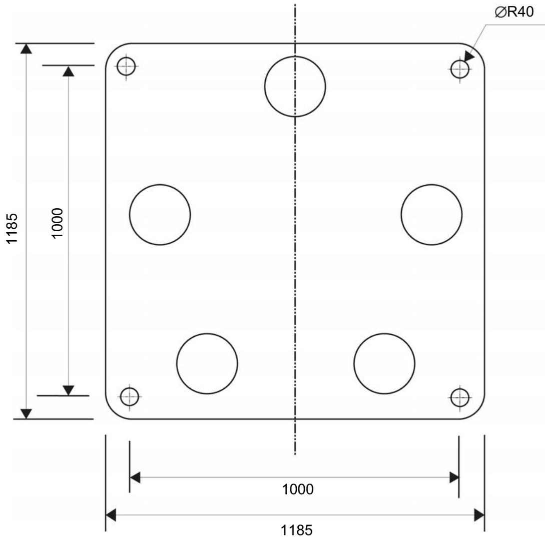
**Figure 1:** CardioWall Compact mounting points
