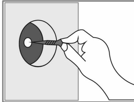
Position appropriate fixings by hand in all corners and tighten with a tool x 4, checking it is level.
